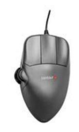
Rubberized surfaces for easier grip with a shape that is molded to fit hands. Multiple sizes and right/left hand orientation available. Scroll wheel and rocker switch located on the side for use with thumb.
