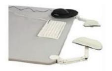
Provides arm support without restricting motion. Includes clamps for work surfaces up to 1-5/8" thick. Provides 17" of reach and 3" of vertical adjustment. Holds up to 35 lbs. \*Tall clamps attack to thick surfaces up to 2-1/2".
